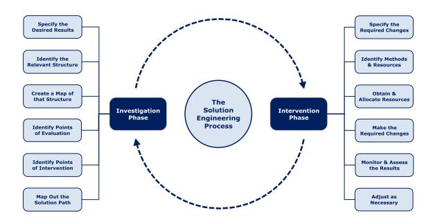
Figure 1 – The Solution Engineering Process
